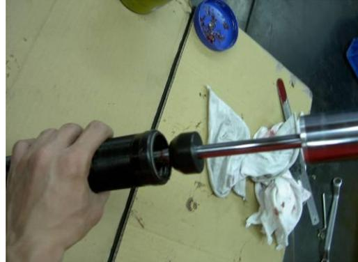
16.) Insert the inner cylinder until the striated tip is through the outer cylinder. Then screw the hex nuts and washer back to original place.
