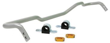
Whiteline adjustable anti-roll bars offer from 2 up to 4 points of adjustment allowing in some cases 10 distinct stiffness settings for precise handling bias adjustment. Bar size (stiffness) also allows for corrections to understeer or oversteer tendencies depending on vehicle type or how the vehicle is being used.
