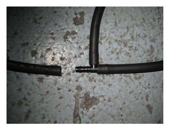
21. To facilitate fitting of the intercooler, we need to relocate the headlight washer tube. Using the supplied silicone hose, connect to the bayonet fitting and plug this in to the passenger washer. Secure it with one of the supplied cable ties. Route the hose as shown below, around the back of the foglight, and clip it in along the bottom of the bumper.
