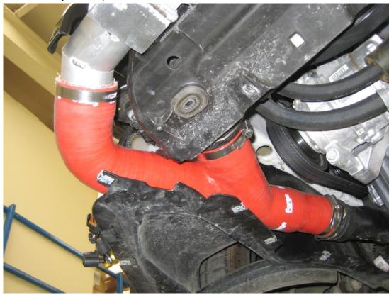
19. Repeat for the passenger side which is easier as there is only one aluminium coupler to contend with. Use a jubilee clip on the end to the intercooler and the end which goes to the turbo. Tighten all the jubilee clips.
