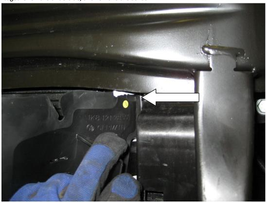
12.On the drivers side, cut out a small section of the lower lip in front of the radiator to assist in fitting the intercooler.
