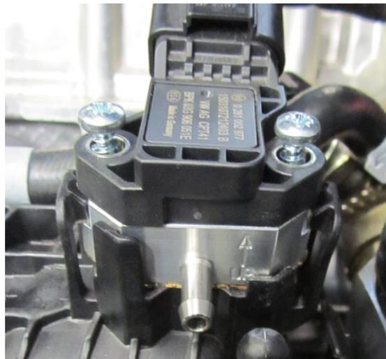
1. Locate the map sensor which is attached to the inlet manifold (circled above). Undo both screws and lift to remove .
