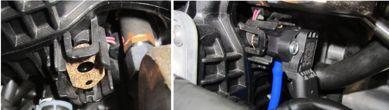
1. Locate the map sensor which is attached to the inlet manifold. Remove both screws (if present), hold back retaining tabs and lift map sensor out.
