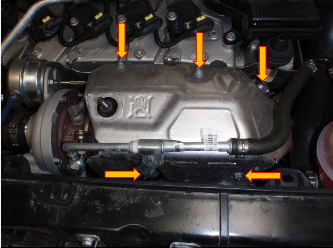
2. With the original heat guard left in place fit the Forge blanket over the top of it. Line up the holes at the top first and using the supplied 3x M6 fasteners and penny washers secure to top half of the blanket, do not fully tighten at this stage.
