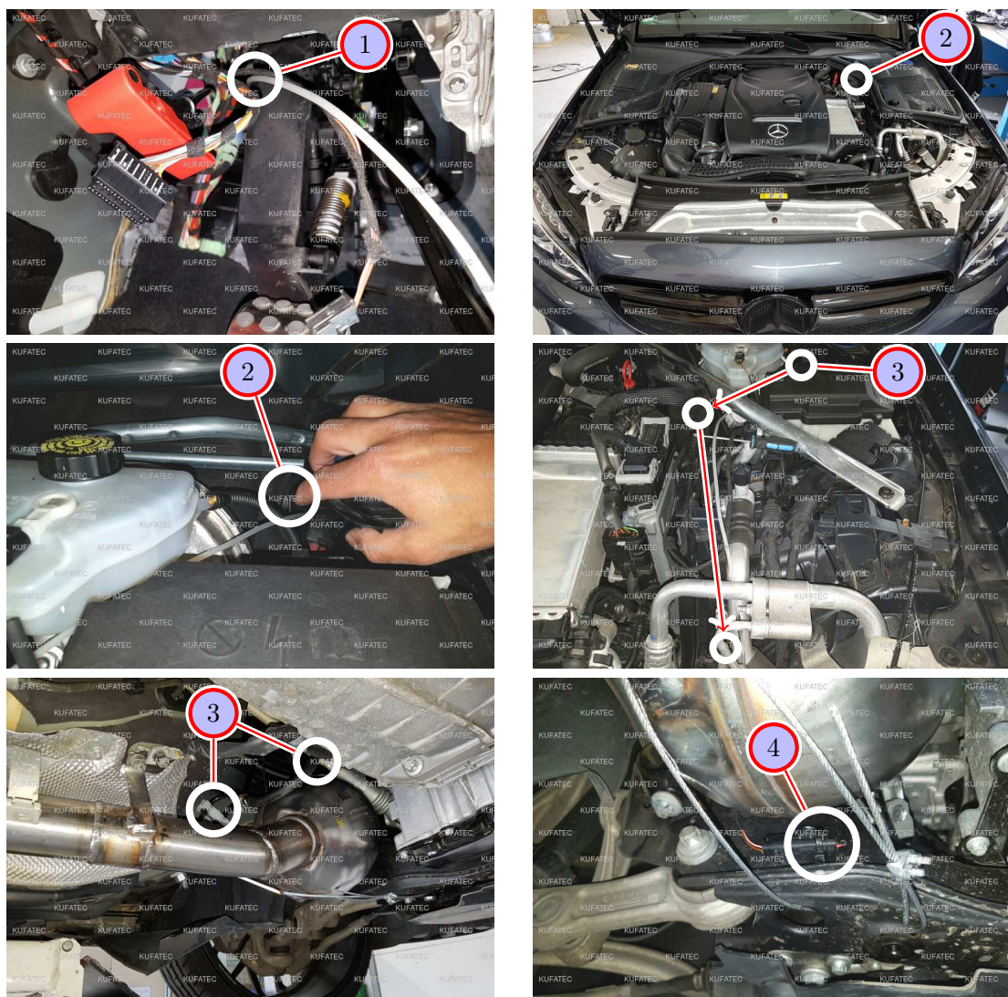
Figure 10: Cable routing to the sound generator for AMG-Line
