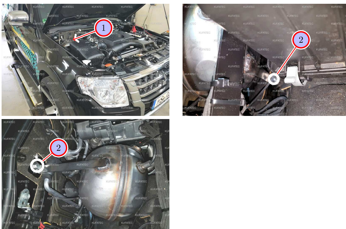
Figure 12: Installation front sound generator
